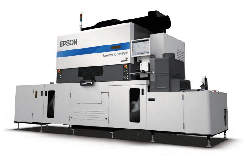
The automated Epson® SurePress L-6534VW Digital Label Press will reliably produce up to 2 million square feet per month\*. The L-6534VW comes standard with White Ink and either digital varnish or Orange Ink, corona treater, web cleaner, ionizer, eye mark sensor and an additional UV lamp — everything required for prime label production. Digital hybrid inline interface is also available.
